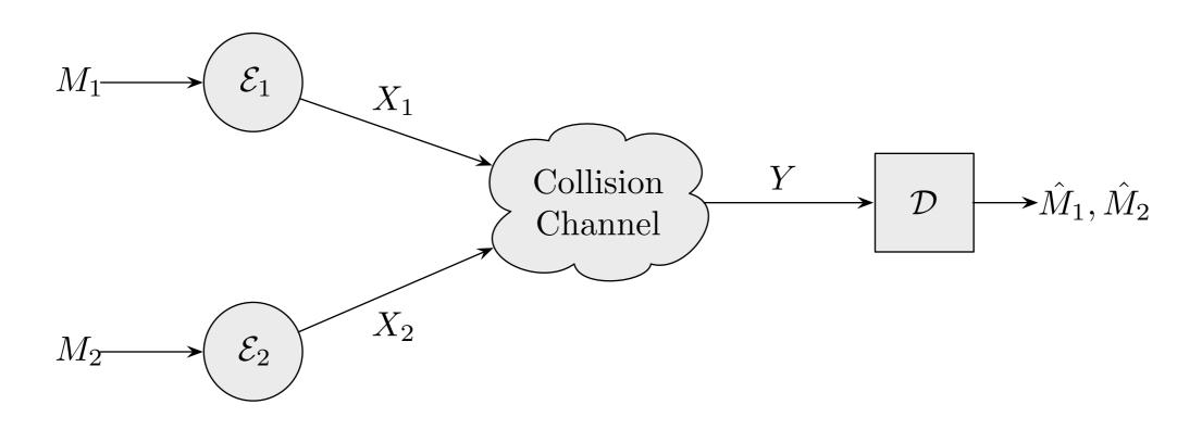
Silent symbol: **S**   $\mathcal{X}_i = \{\mathbf{S}, x_i(1), x_i(2), \cdots, x_i(q_i)\}, i \in \{1, 2\}$ Collision symbol: **C**  $\mathcal{Y} = \mathcal{X}_1 \cup \mathcal{X}_2 \cup \{\mathbf{C}\}$
